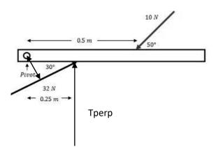
Torque can be thought of as a "turning force". It tries to cause things to rotate. Any object that is not moving is in what we call static equilibrium. To be in static equilibrium there are 3 things that must be true.
