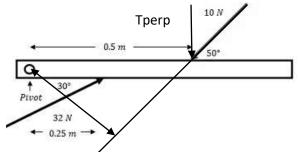
Extend the force. Then draw a line perpendicular to it to the pivot. Calculate this line "r".
