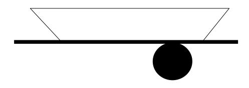
a. The boat has an outboard motor weighing 90 kg is fitted to the back of the boat 1.15 metres behind the axle. What is the force acting on the tail bar? [6 marks]
