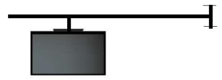
a. If the screen is 70 cm from the wall and the 2 bolts are each 5 cm from the metal bar calculate the horizontal force in each bolt. [6 marks]
